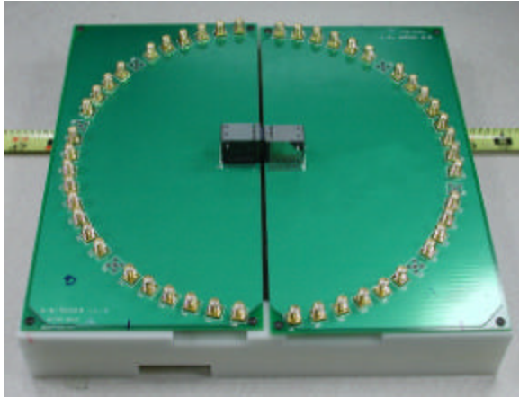
Top View of Crosstalk Test Setup - Road Runner
